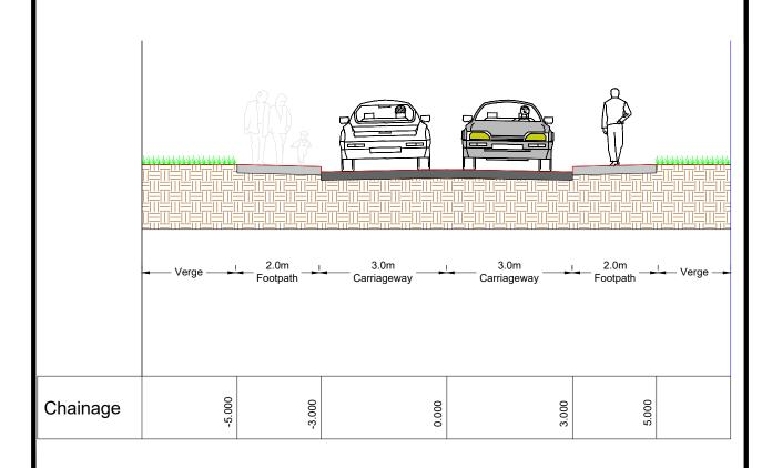
Typical Cross Section - Estate Road (Footpath on Both Sides)
