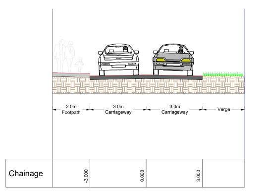
Typical Cross Section - Estate Road (Footpath on One Sides)
